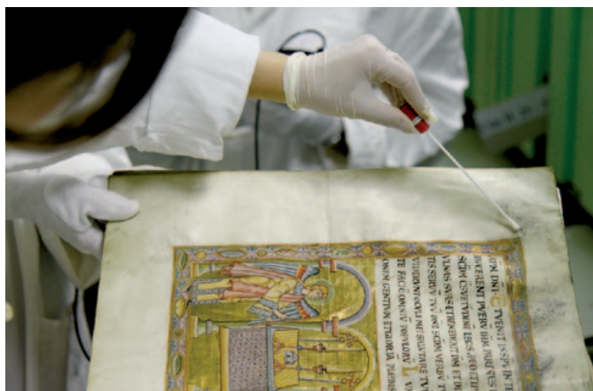
The testing of the microbiological activity in the Vyšehrad Codex. Photo: Petra Vávrová
